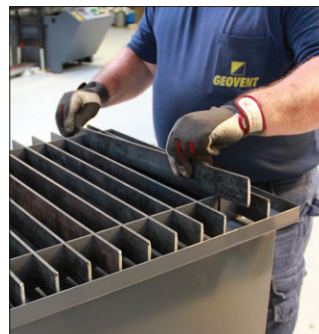
The rods can easily be moved / changed if needed.
